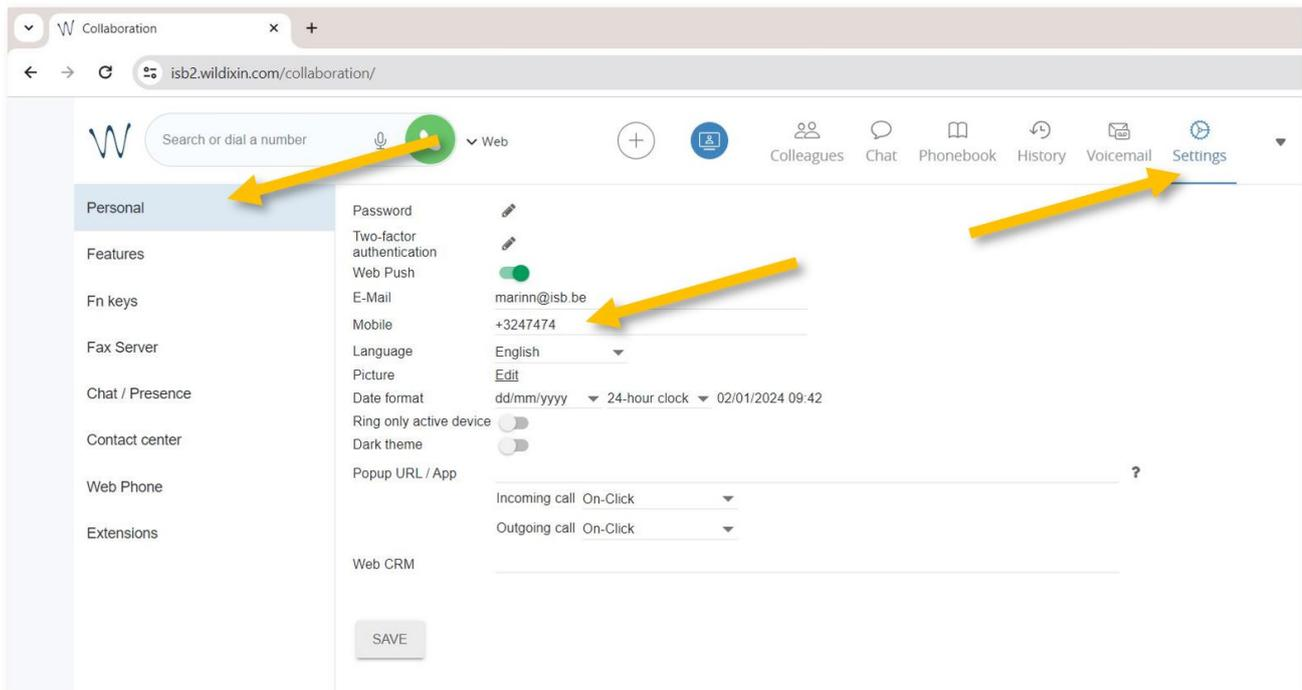
Then select the Features tab and activate the Enable mobility with timeout. In the example underneath, the default (10) was changed to 2, meaning that after 2 seconds, the mobile phone and the computer (if logged in to Wildix) will also ring.
